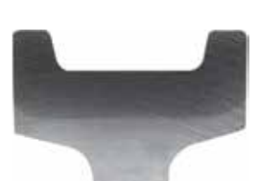
AISI-4140 Super Tough Wheel Section (Based on a 24" Wheel Sample)
