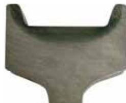
Differentially Hardened Wheel Section (Based on a 27" Wheel Sample)
