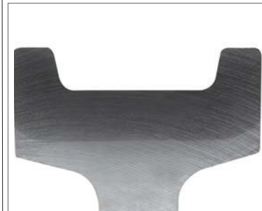
AISI-4140 Super Tough Wheel Section (Based on a 24" Wheel Sample)
