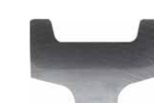
AISI-4140 Super Tough Wheel Section (Based on a 24" Wheel Sample)
