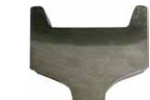
Deep Hardened™ Wheel Section (Based on a 27" Wheel Sample)
