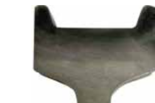
Rim Toughened Wheel Section (Based on a 27" Wheel Sample)
