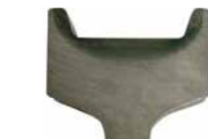
Differentially Hardened Wheel Section (Based on a 27" Wheel Sample)
